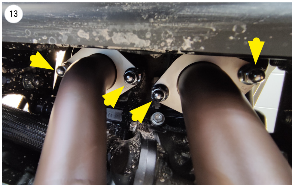
install the primary pipe
