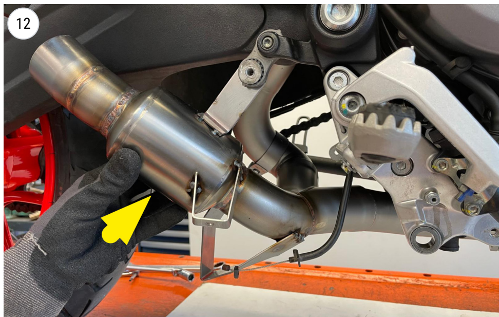
Install the pipe
