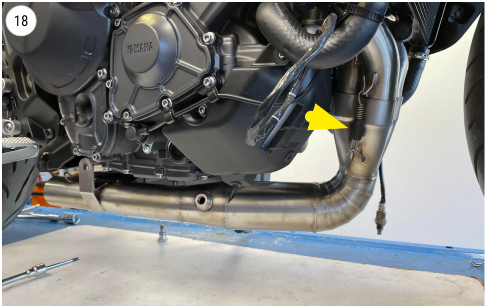
fit the secondary pipe and hang the spring
