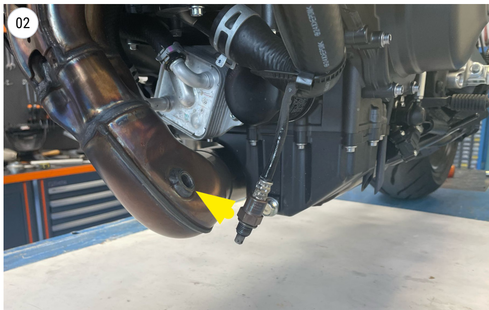
unscrew the sonda lamba / O2 sensor
