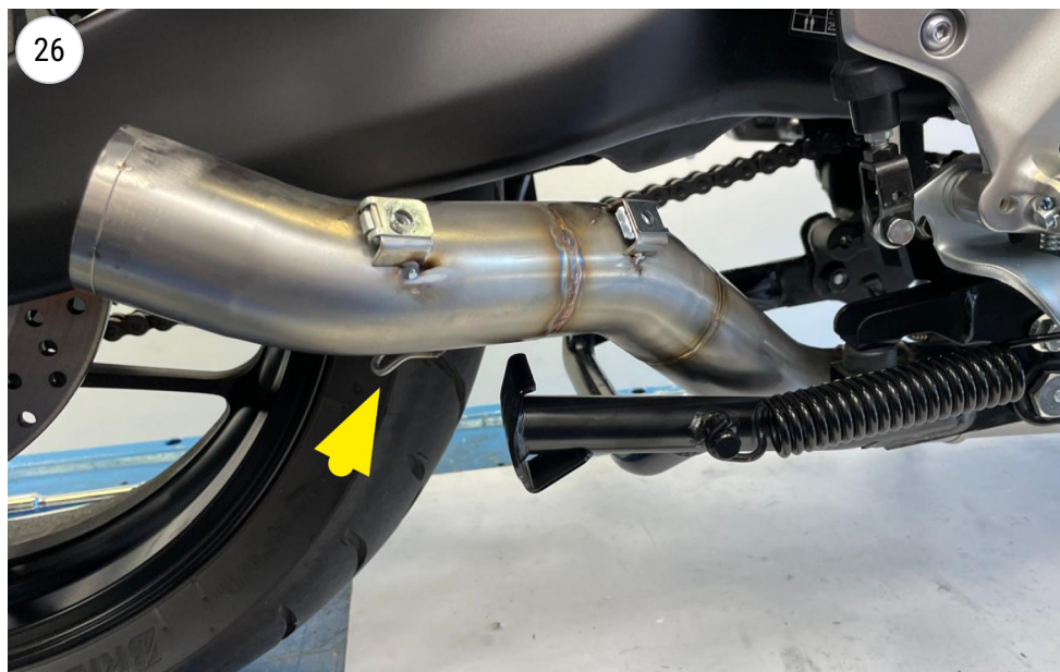
fit the final pipe
