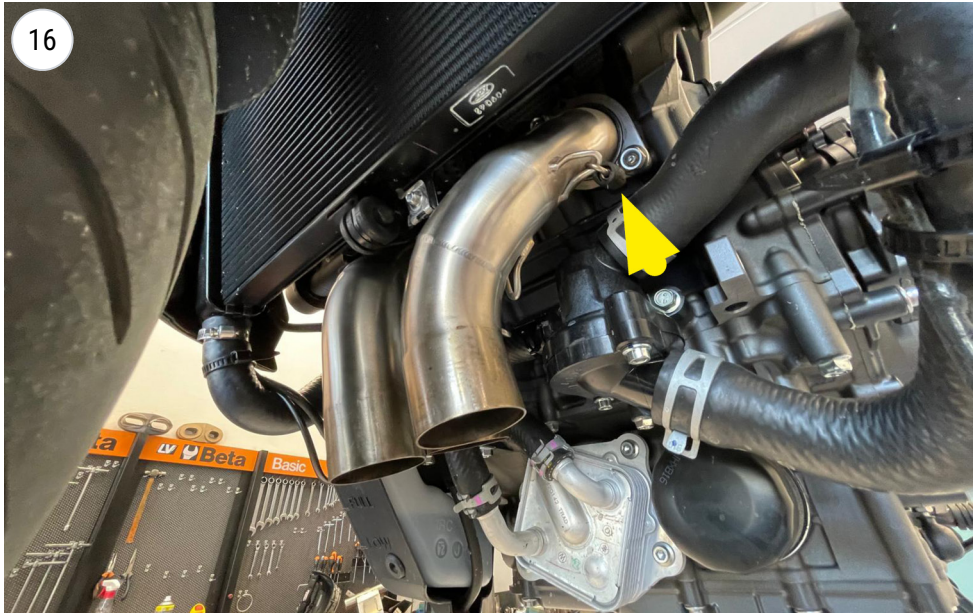
install the primary pipes and hang the spring
