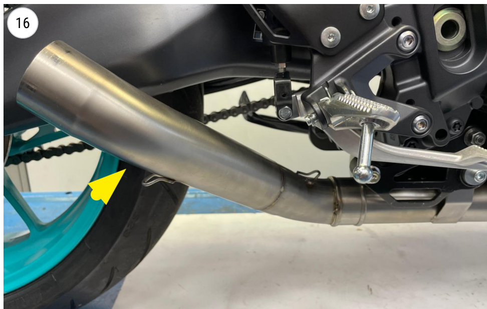
install the final pipe
