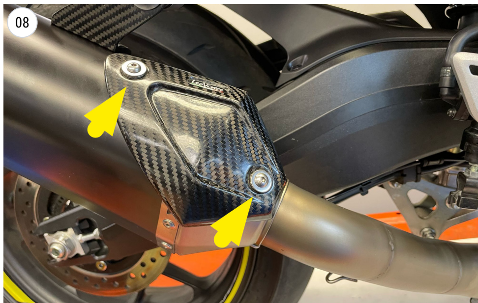
install the carbon heat shield
