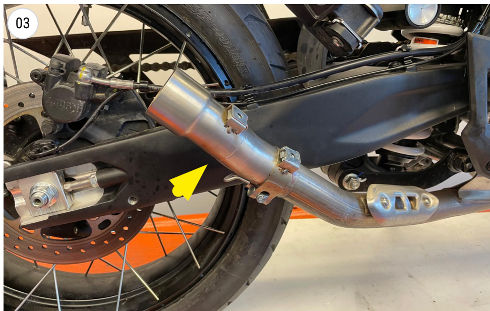
install the pipe with the clamp
