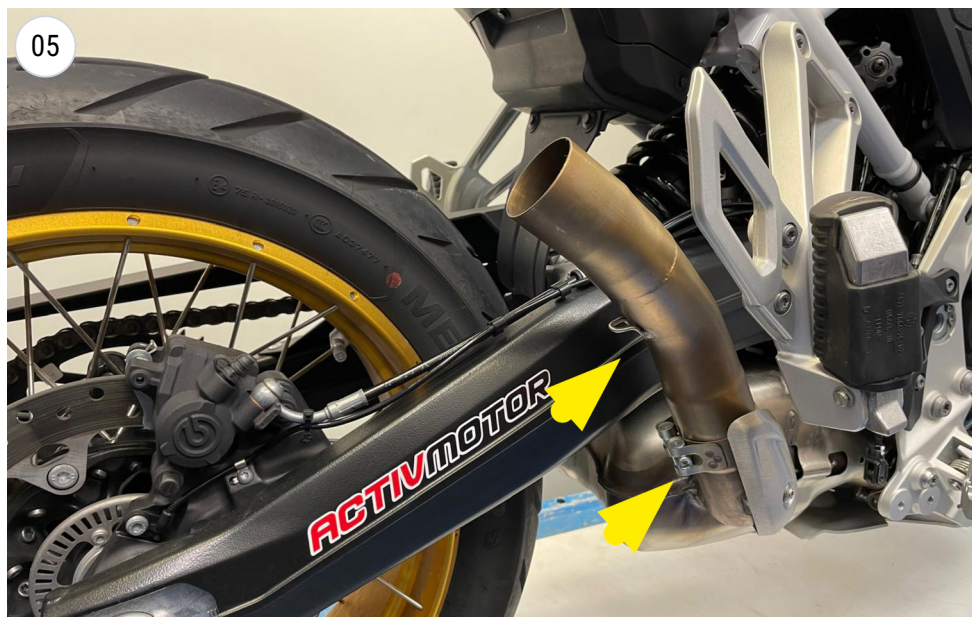
fit the pipe with the clamp
