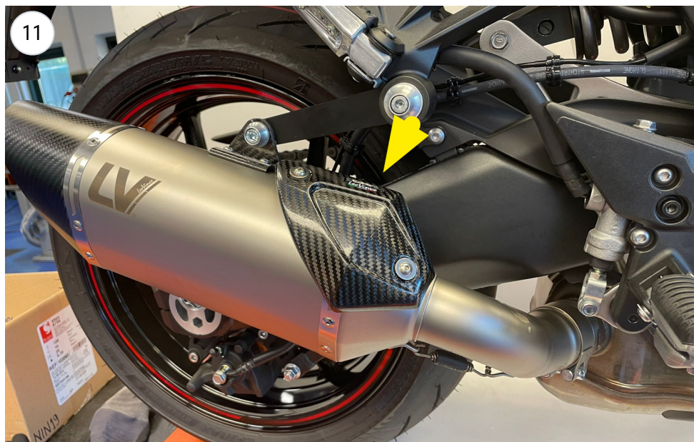
FIT THE LEOVINCE CARBON HEAT SHIELD
