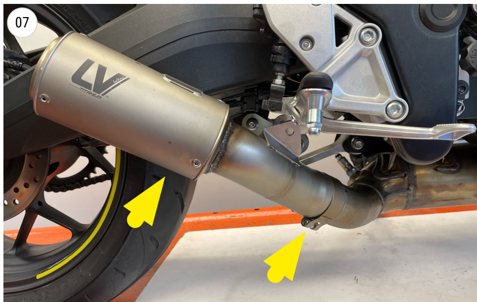
fit the muffler with the clamp
