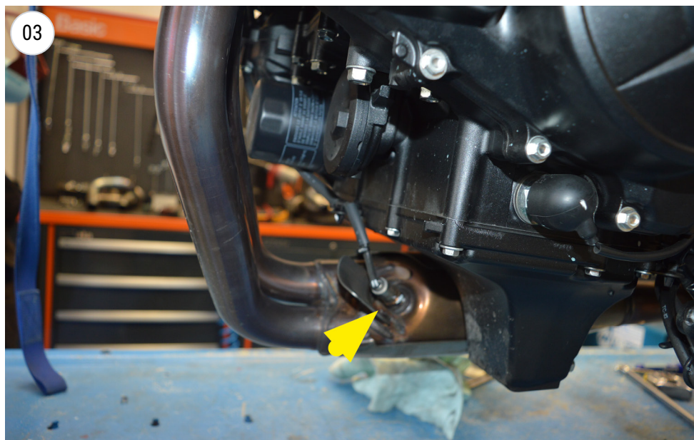
remove the Lambda/Oxygen sensor
